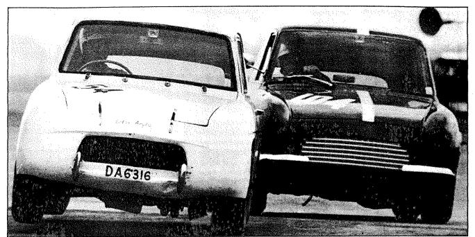
nal block - that one has proved untraceable), 45DCOE Weber carbs, highly modified heads and cams, early Elan gearbox, 4.125 ratio limited slip diff, Cortina brakes (state of the art back in 1965) drilled for ventilation, Consul 315 front suspension with chopped Zephyr springs, Panhard rod rear suspension, Cosworth dry sump in boot cavity, oil cooler in front of radiator, estimated output about 180bhp.
